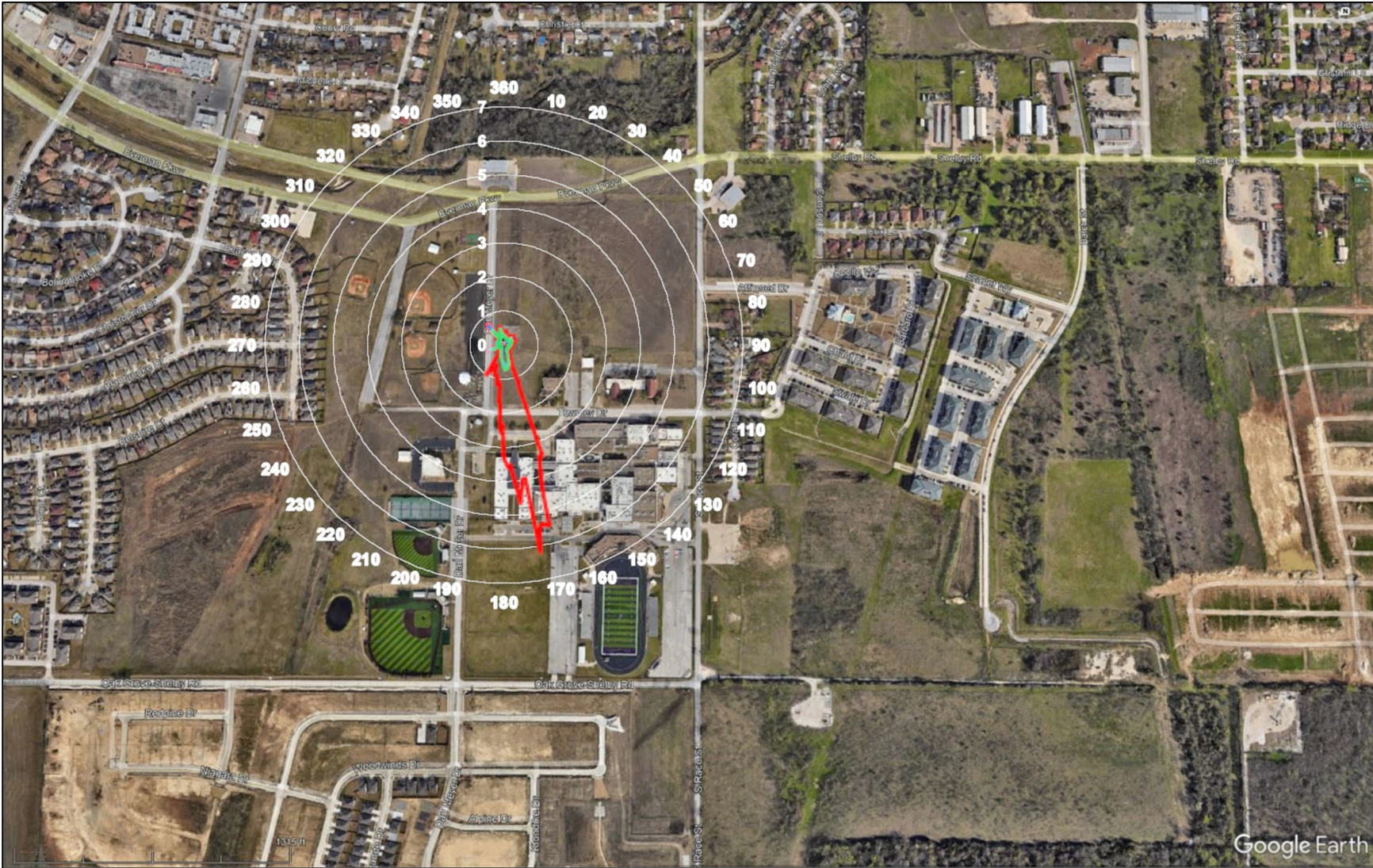
Figure 3-11. Everman Johnson Park Toluene Pollution Rose (ppbv) for June 2023 – August 2023 Overlain on Map of Site Area
